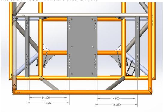
1.5) Install the 1141-12 bracket to the 1101-06 chassis cross tube. The 1141-12 bracket should fit inbetween the 1103-13 and 1103-06 tubes with small gap on either side. Orient the front face of the 1141-12 vertical to the chassis or the top face horizontal. One of the main chassis tubes like 1100-02 or 1101-03 is a good reference. Tack weld in place
